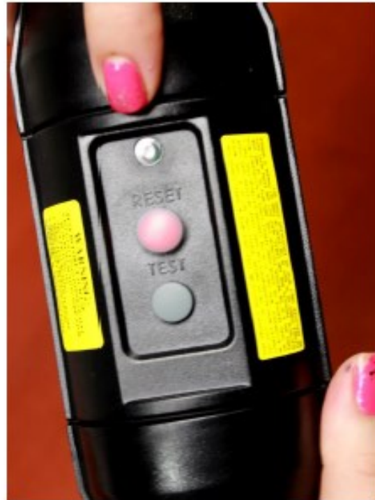
3.) Check GFCI, and push "reset" if necessary.
